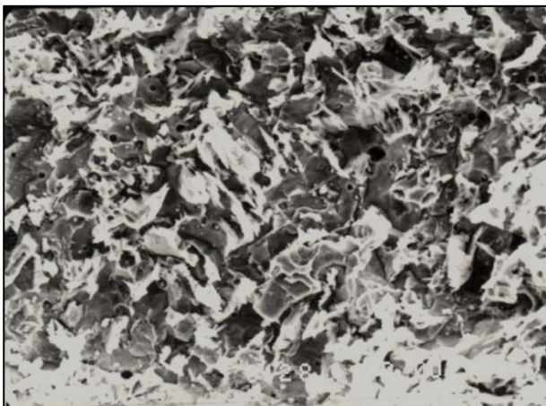
Fig. 6. Microstructure of martensite and residual austenite of reinforcing steel (x600)
